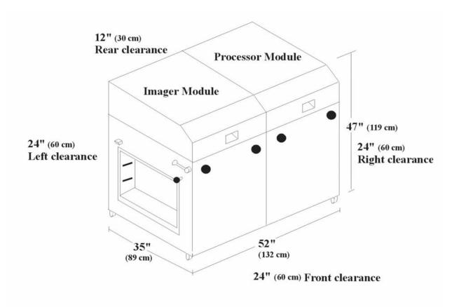
A 9-foot (2.7 m) power cord is supplied with the PlateStream. It is attached near the Power Switch. A 220-240 V male connector is required (to be supplied by the customer). It will be wired to the power cord to mate with the customer's 220-240 V female outlet.
